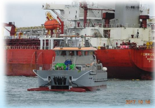
Drill of oil spill collection by the vacuum drainage system of the Mailiao Marine
