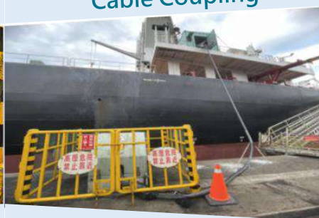
Ship-to-Shore Cable Coupling
